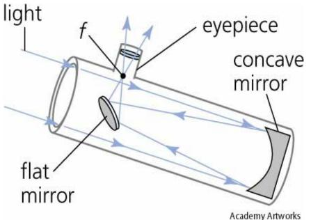
Telescopes an optical instrument designed to make distant objects appear nearer, containing an arrangement of lenses, or of curved mirrors and lenses, by which rays of light are collected and focused and as a result this tool lets mankind look beyond earth into the heavens. Therefore telescopes have given us a new understanding of our place in the universe and continue to show us new exciting
