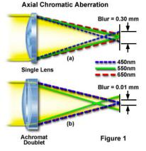
As light passes through a lens, it breaks up into various colors because the glass bends the colors by different amounts. Newton's solution was simple: He took the lens out of the telescope. Newton replaced the primary lens with a polished, rounded, metal mirror. He experimented with different mixtures of metal and decided on one that was six parts copper to two parts tin. It was almost as bright as expensive, quick-tocorrode silver and would reflect a lot of light.
